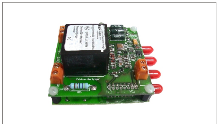
Intrinsically safe Profibus modem for RS485, RS232, BB 22444, fiber optics etc.
